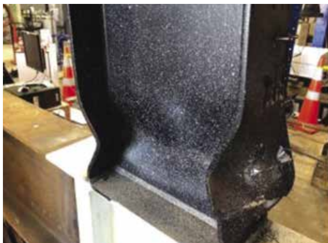
This figure from HERA report R8-43 illustrates the failure of a specimen following cyclic loading in the lab.
