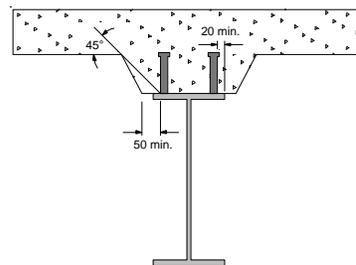
Figure 2: Haunch Detailing
