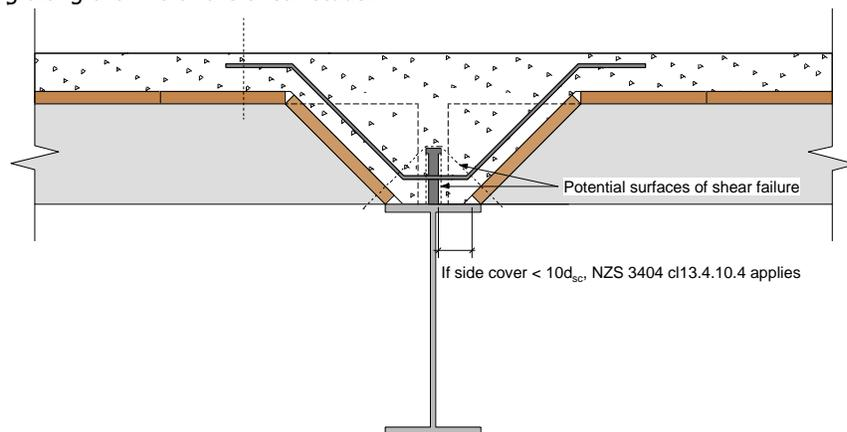
Figure 3: Typical potential surfaces of shear failure (topping reinforcement not shown)
