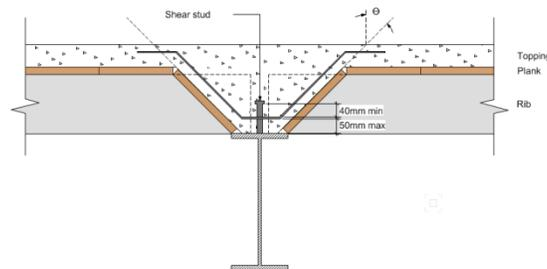
Figure 1: Cross section – composite steel and precast ribbed floor
