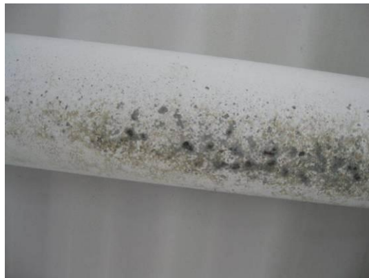
Figure 18. Failure of Duplex TSZ
