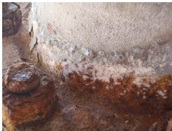
Figure 20. Hydrogen bubbles from duplex TSA
