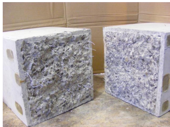
(b) SFRC specimen after direct shear test
