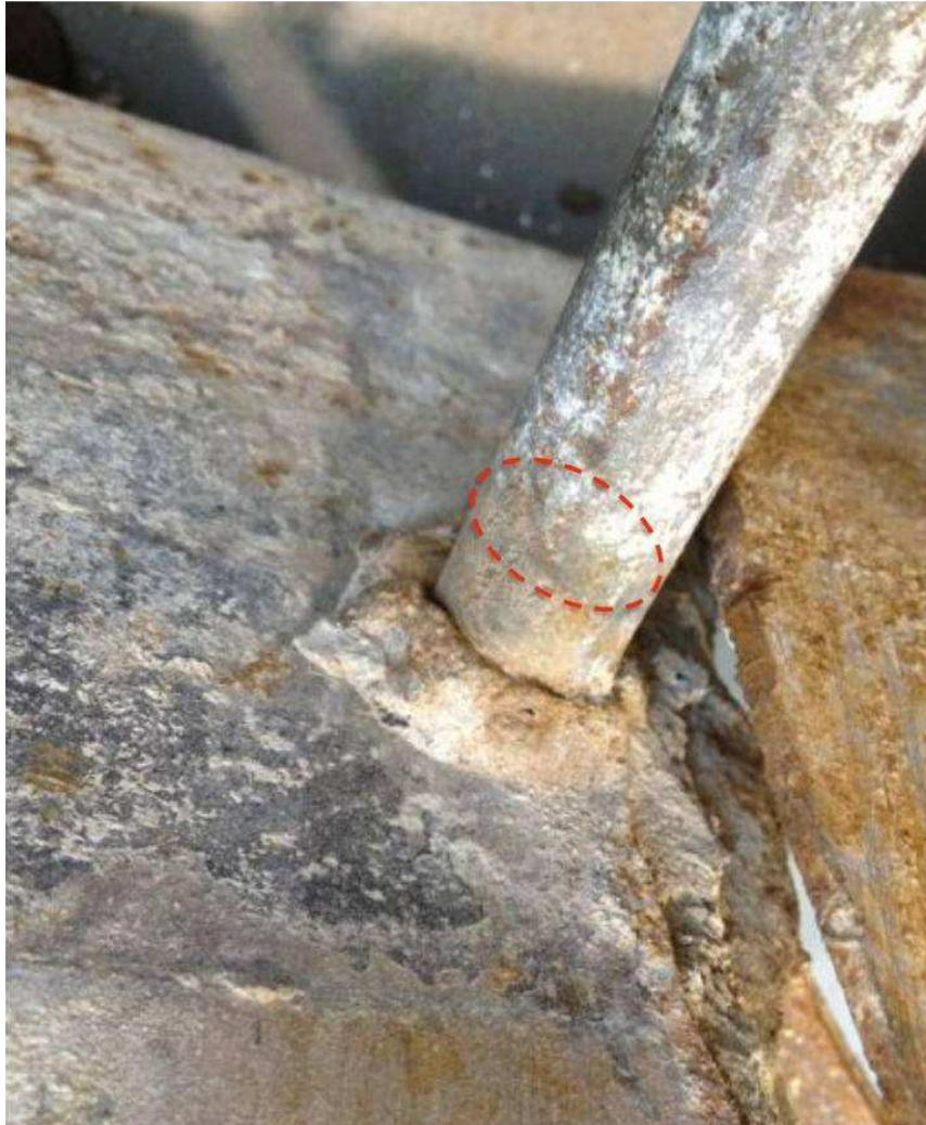
Figure 4: Link fracture adjacent to shear stud. Image courtesy Milo Kral, University of Canterbury
