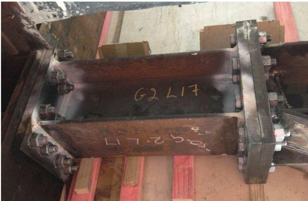
Figure 10: Bolted-in active link. Image Spiire New Zealand Ltd.
