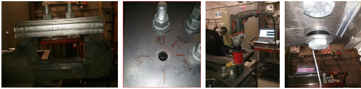
Figure 4: Bolt tightening test setup (a), Measuring the nut turn (b), The torque wrench to apply the part turn (c), and The load cell (d)
