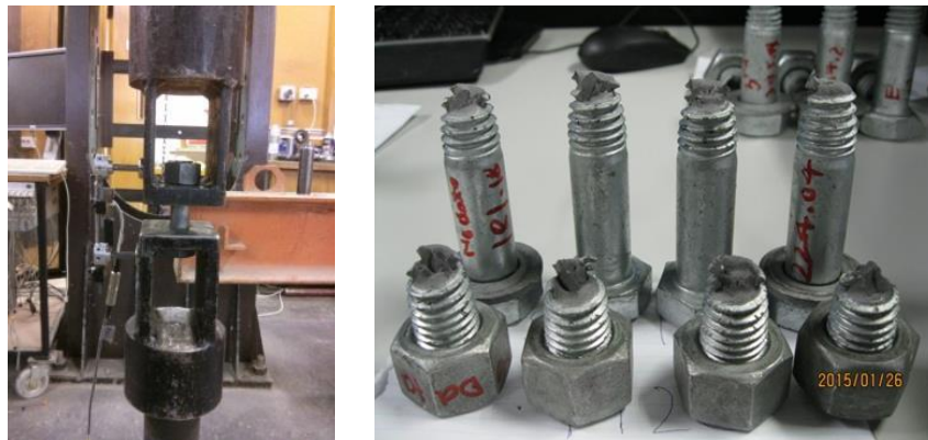
Figure 1: Bolt tensile test on 500kN MTS (left) and Fracture surfaces of the tensile tested bolts (right)
