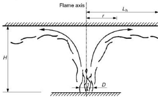
Figure 4: Localised fire – for flames which impinge on the slab /beam above
