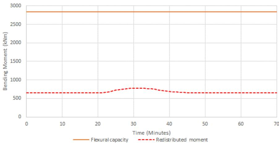
Figure 12: Comparison of flexural capacity and applied bending moment for each secondary beam located 3.8m from the fire location.
