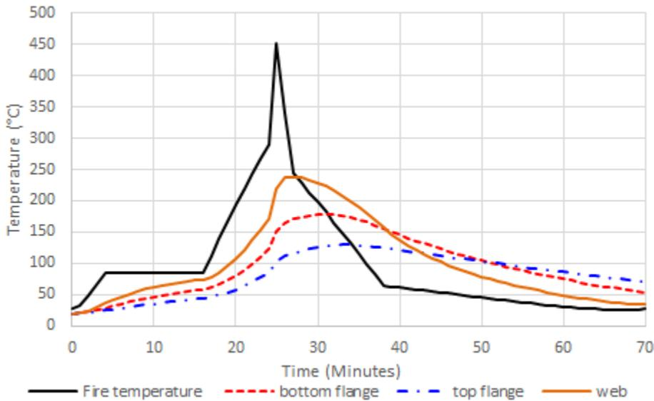
Figure 11: Calculated steel temperatures of beam located radially 3.8m from fire.
