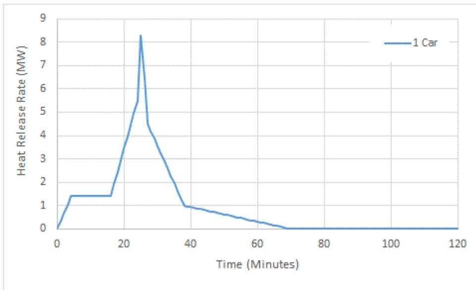
Figure 2: Design HRR curve for a single car fire – Sprinklered carpark
