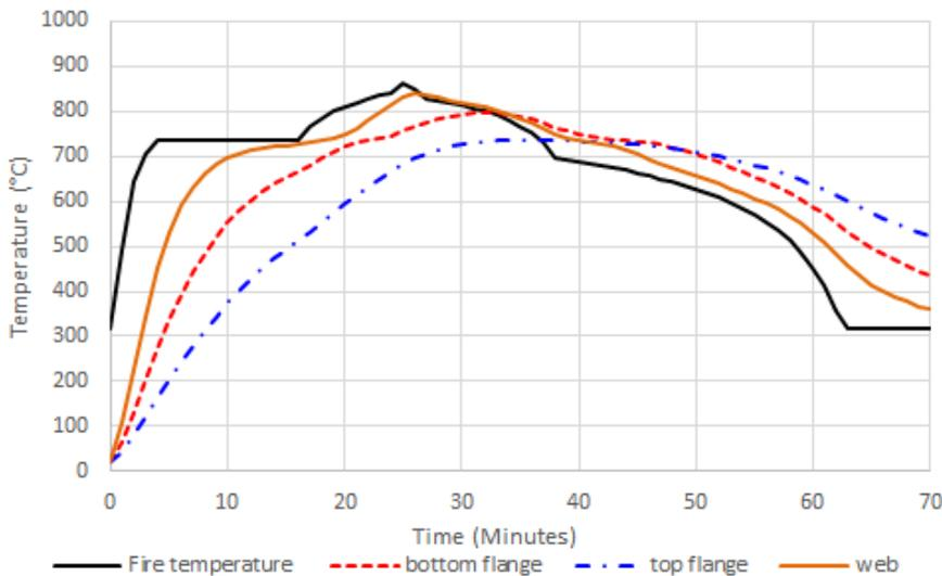
Figure 7: Calculated steel temperatures of beam located directly above the fire.
