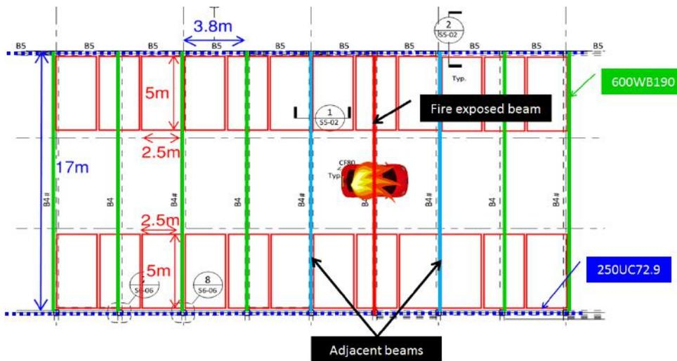
Figure 10: Location of adjacent beams relative to main fire-exposed beam.
