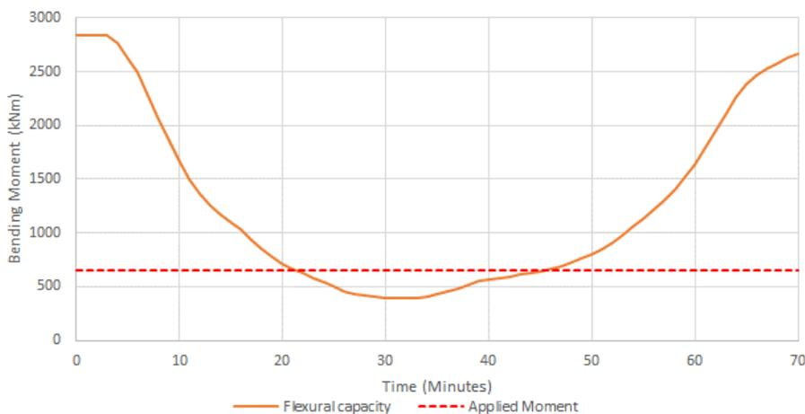
Figure 8: Comparison of flexural capacity and applied bending moment
