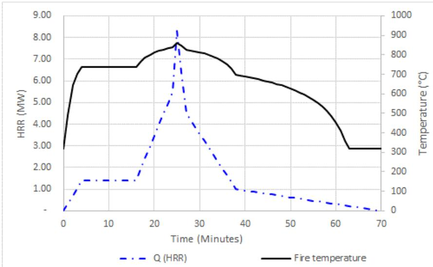
Figure 6: Calculated fire temperature above at the soffit of beam above the fire.
