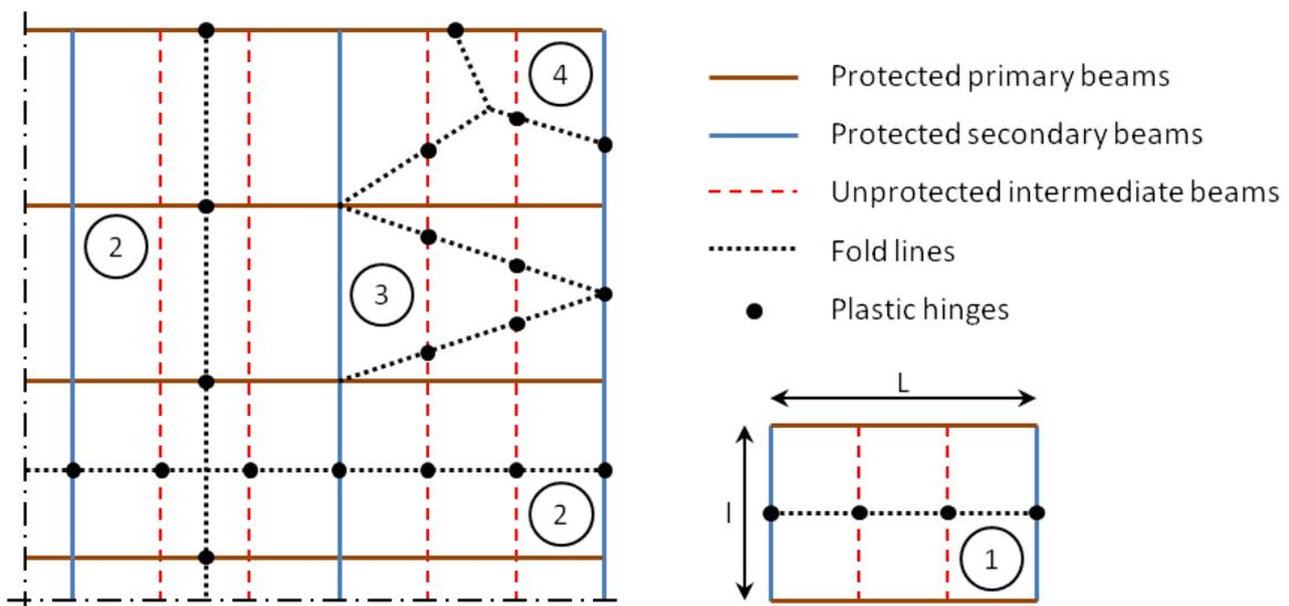
Figure 2. Proposed collapse mechanisms
