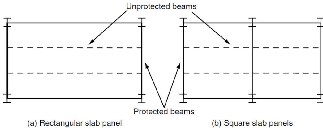
Figure 1. Rectangular and square slab panels (Abu et al., 2011)
