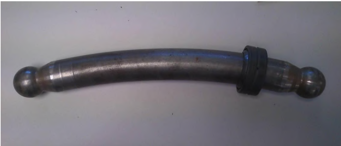
Figure 2. Yielded pin after testing.
