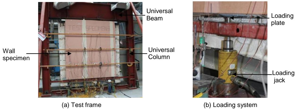
Figure 5. Test Frame and the loading system
