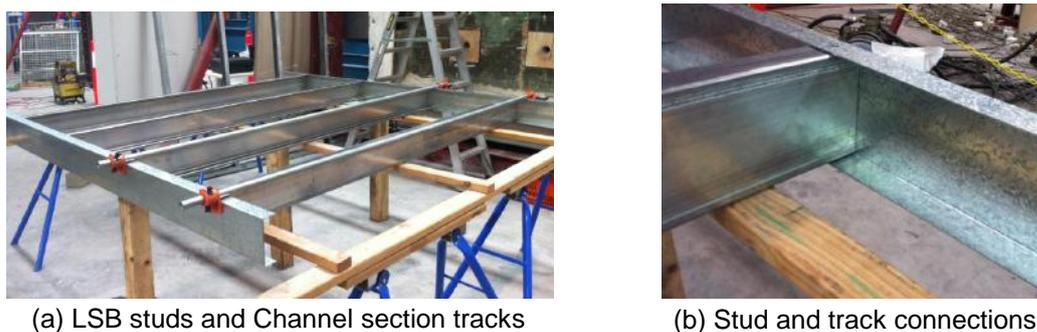
Figure 2. Fabrication of test specimen
