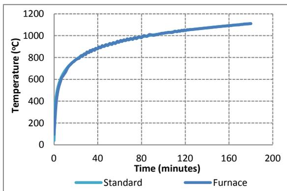
(a) Standard curve versus Furnace temperature
