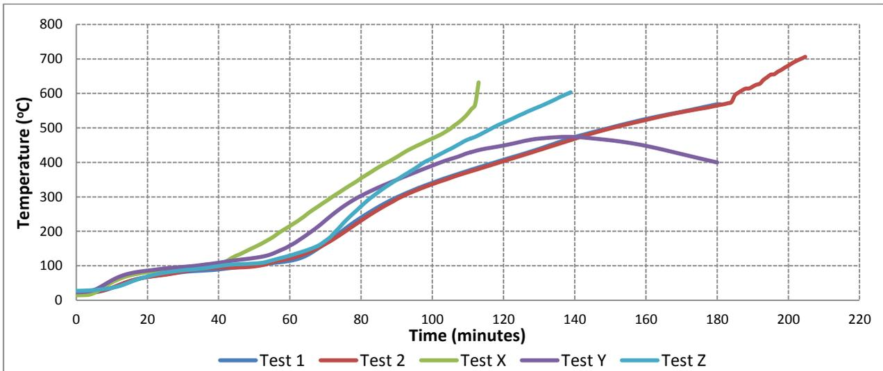
Figure 12. Hot flange temperature of failed studs
