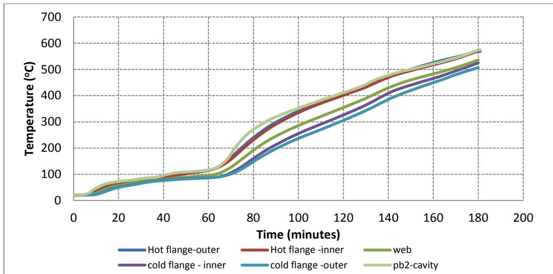
Figure 8. Time-Temperature profiles of the steel stud surfaces with time in Test 1
