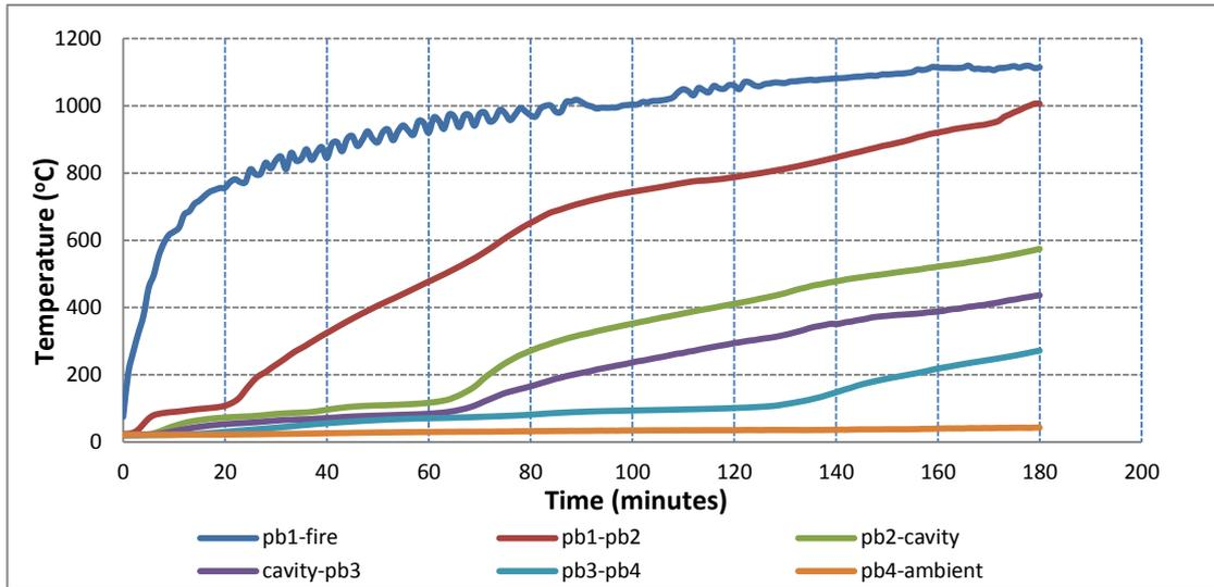
Figure 7. Time-Temperature profiles of the plasterboard surfaces in Test 1
