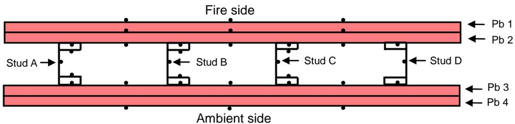
Figure 4. Locations of thermocouples
